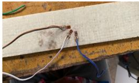
Figure 2: X, Y, Z axis Strain gauge Attached with Composite laminate
