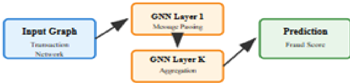
Fig. 2. General architecture of GNN-based fraud detection showing message passing, aggregation, and prediction.
