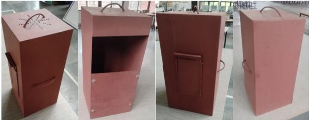
Figure 4: Designed heat recovery structure using CRC sheet with red oxide coating
