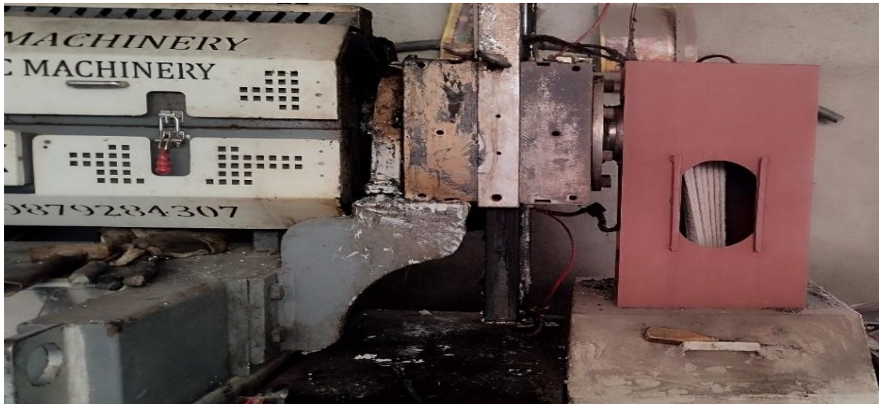
Figure 5: Assembled view of mother unit, heat recovery structure and baby unit (integrated setup)
