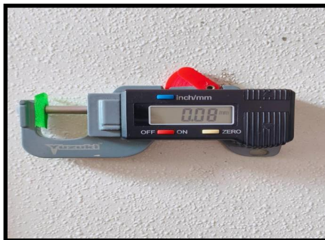
Fig No2: - Thickness of mouth dissolving film
