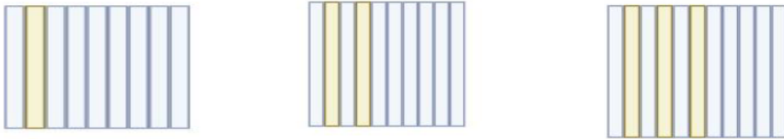
Figure 8: Schematic representation of the structure of the samples made of 8 sheets of PLA. a) 8 PLA + 1 Lanolin, b) 8 PLA + 2 Lanolin, c) 8 PLA + 3 Lanolin
