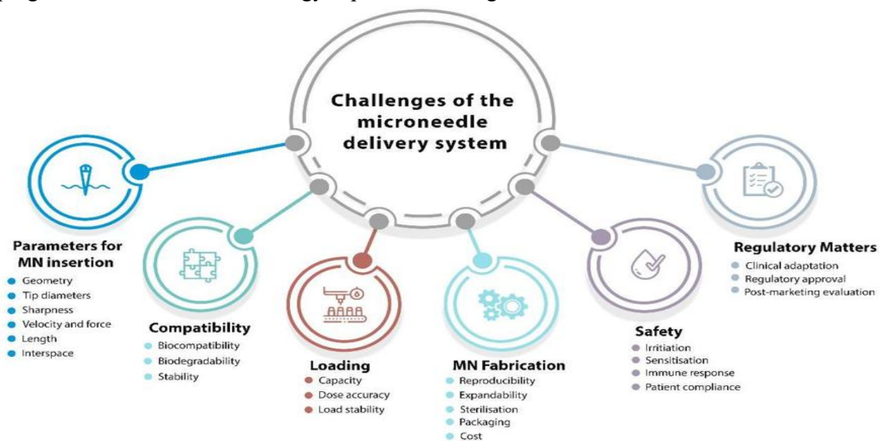
Figure 3. Factors effecting development of microneedle-based delivery system.
